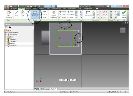
15. Click on Dimension. Hover over the right side of the 2-point rectangle you created until it turns grey and shows a small double arrow, then click and move the mouse to the right until you see the measurement/dimension displayed, then click to place it. Edit the dimension to 1. Then Dimension the lower right hand part of the smaller square to be .5 from the right and .5 from the bottom. Then click Finish Sketch.
