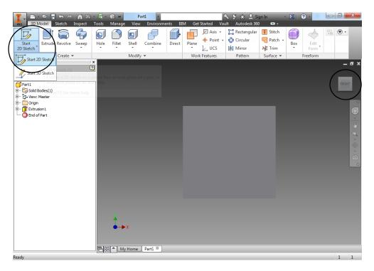
11. Place a Point (plus sign +) in the middle of the box. If you hover slowly you will see the X and Y axis display as 1.000 with two little dotted black lines. Click to place the point (which will be exactly in the center).
