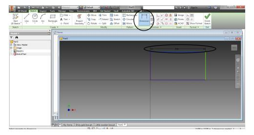
Click on the side of the model that you want to dimension and pull the dimension bar out. Click again to place it and have the box open to input the dimension you want.
